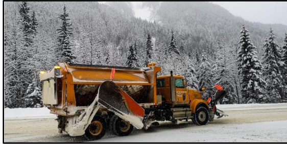
Figure 8. Tandem-Axle Truck with a Wing Plow, Underbody Plow, Front Plow, and Hopper.
